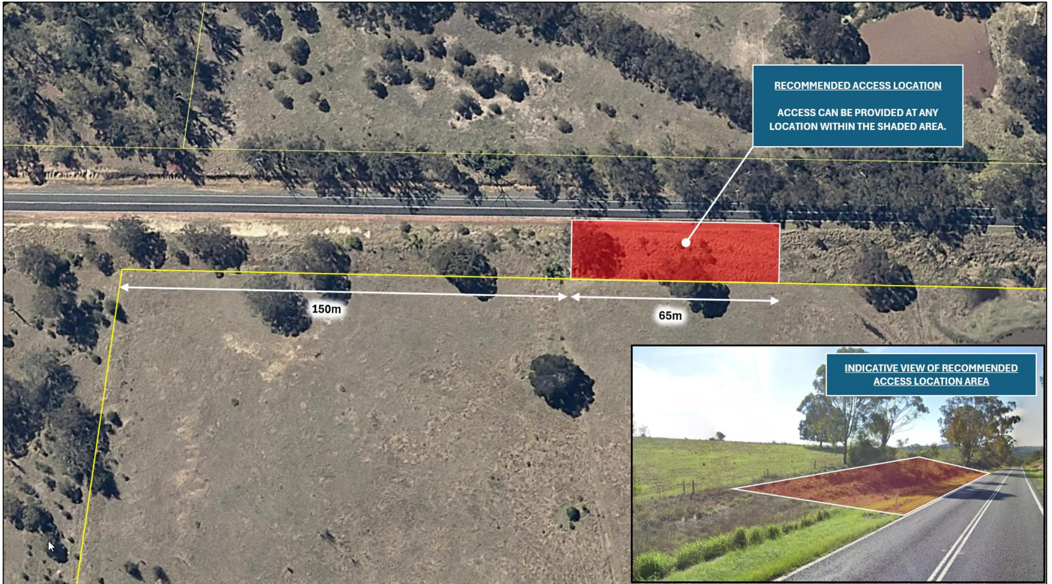
Figure 9: Recommended access location (Ch. 56.330km – 56.380km)
